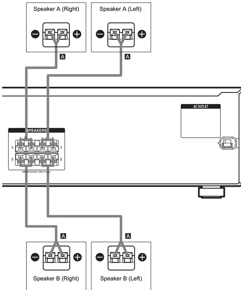
\* If you have an additional speaker system, connect them to the SPEAKERS B terminals. You can select the speakers you want to use with the SPEAKER A and SPEAKER B buttons. For details, see “Selecting the speaker system” (page 17).
