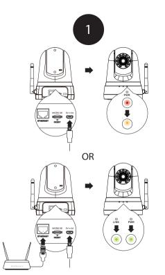
Wireless set-up: Plug the included USB Power Adapter into the back of the camera. Wait until the PWR LED changes from red to blinking orange.
