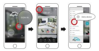
New users: Tap **Sign Up** to register for a mydlink account, then tap Add a Device to install your camera. Existing users: Sign In using your mydlink account and tap the icon at the top left, then tap **Add a Device** to start the setup wizard.
