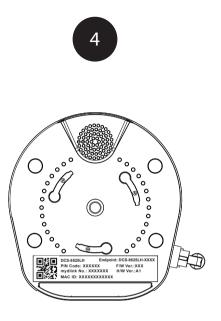
When asked to scan the Setup code, use the code found on the bottom of the camera.
