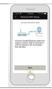
6. Ensure an Ethernet cable is connected from the router to the camera and the included power adapter is connected to the device. Allow the device to initialize (if applicable) and press **Next** to continue.
