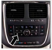
Heated Steering Wheel Switch Location
