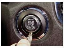
**ENGINE START/STOP Button Removal**
