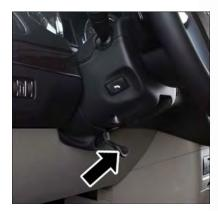
Tilt/Telescoping Steering Column Lever
